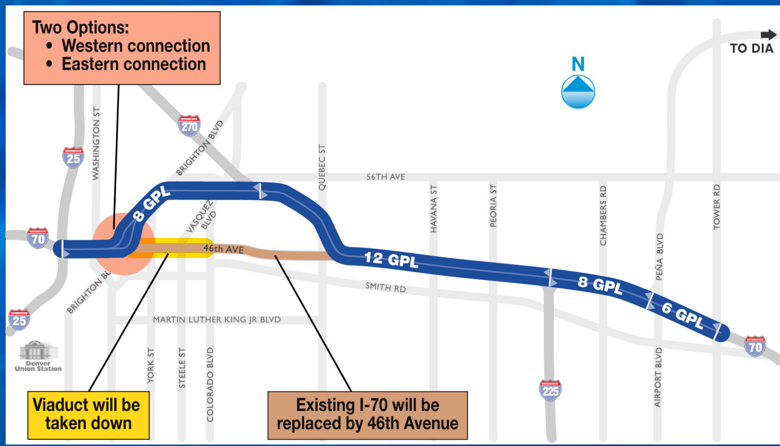
Realignment with general purpose lanes
